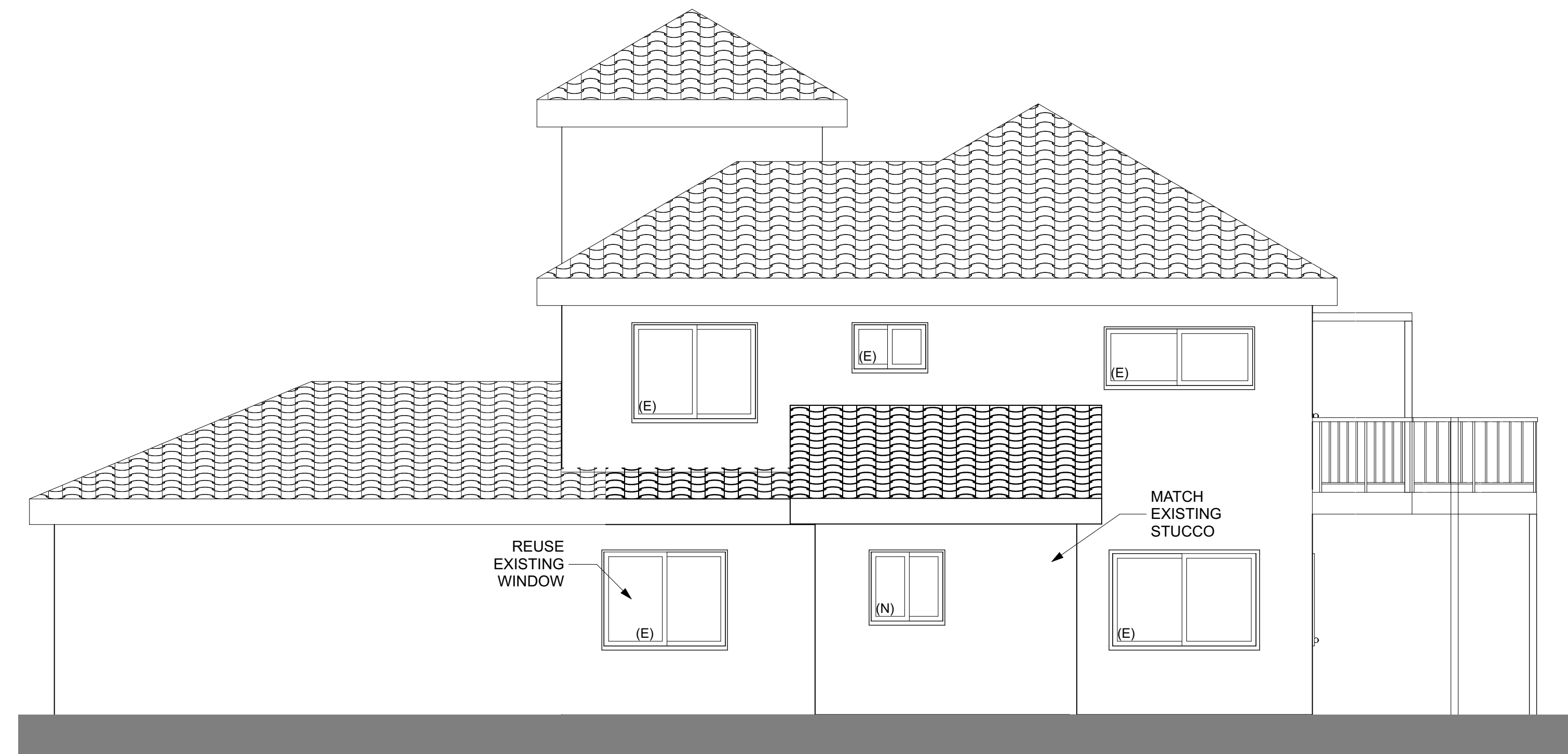
North Elevation SCALE: 1/4" = 1'-0"
